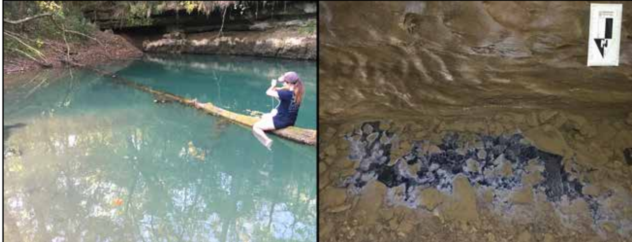
Figure 2 (left): Sarah Burgess sampling sulfide at Orangeville Rise using a syringe, a two-way valve, and a bottle containing a zinc acetate solution. Figure 3 (right): Sulfur seep found near the Second Discovery in Bluespring Caverns. The black residue is from organic matter while the white haze is created by sulfur oxidizing bacteria.
